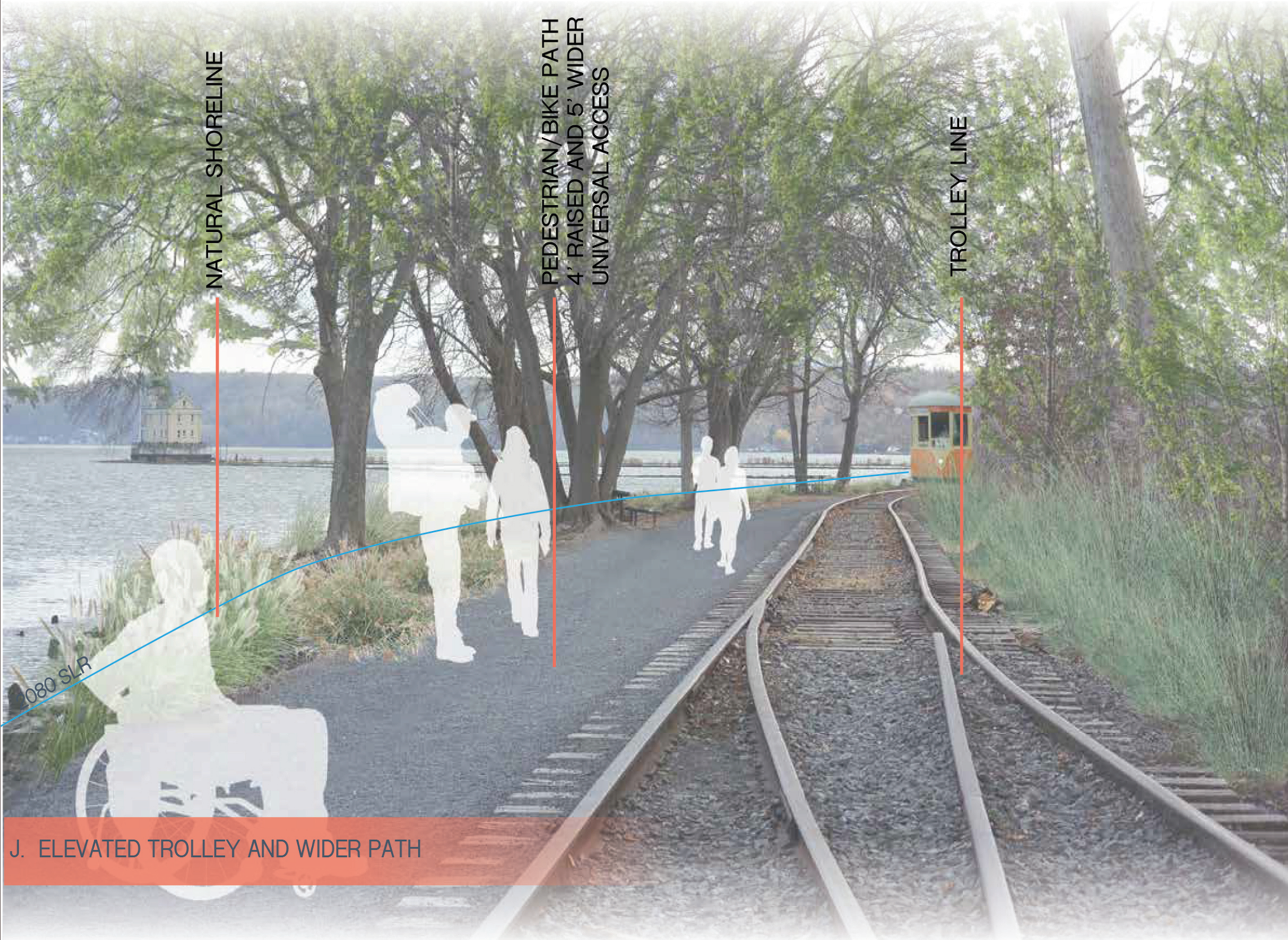
Raising the current trolley tracks 4 feet will allow the trolley to continue operating through 2080 with expected sea level rise. Widening the path along the tracks will allow for more utilization of the path.
