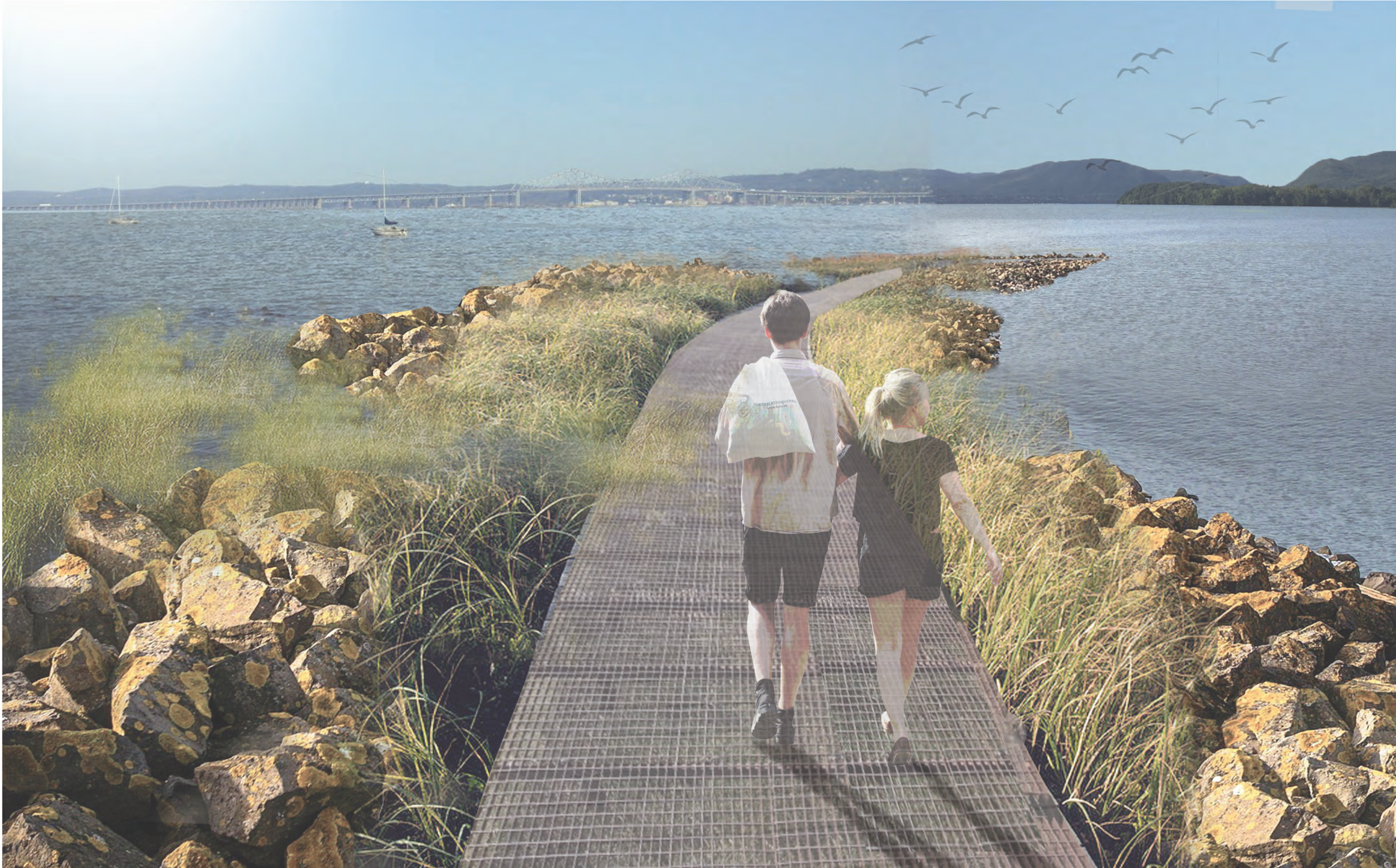
Northern pier ecological buffer and pedestrian walkway to protect Piermont agaisnt wave action and reduce sediment deposition
