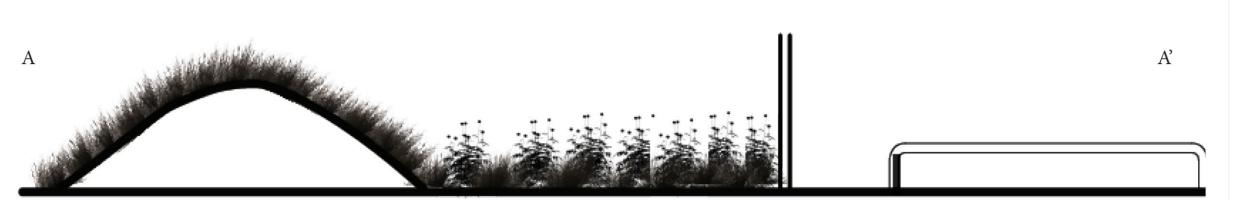
Gas Works Berm - As with the Waste Water Treatment plan, our intention is to preserve this piece of infrastructure with an economically viable intervention. This berm is built to four feet high which should provide protection from sea level rise projected at 2080.
