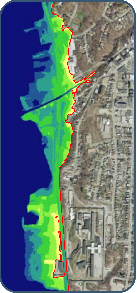
Inundation depths (blue) and temporary flooding depths (green) for the “100-year” or 1% flood on the Ossining waterfront with 60” of projected sea-level rise, which could occur as soon as the 2080s, according to NYS official projections.
