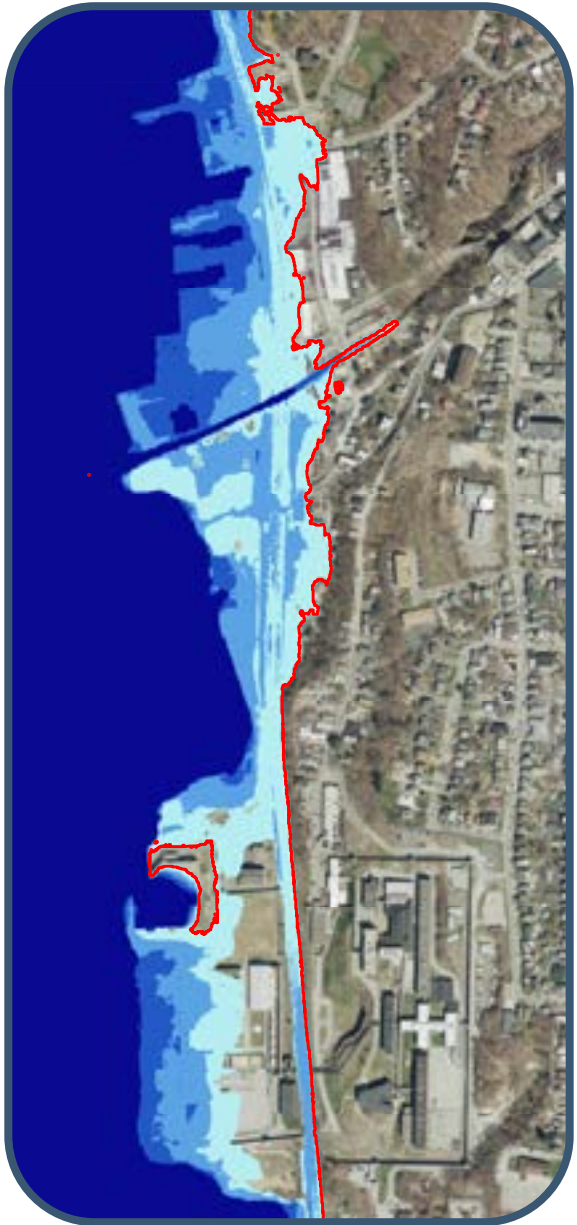
Ossining's waterfront provides an example of increasing flood risk in many Hudson River towns. Depths of temporary flooding from the “100-year” or 1% annual chance flood for the 2020s baseline condition. Darker blue = greater depth.
